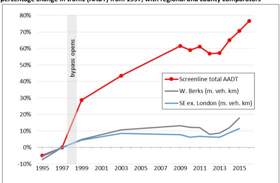
Figure 7.3: Screenline across A34 Newbury Bypass and A339 bypassed old road showing percentage change in traffic (AADT) from 1997, with regional and county comparators
