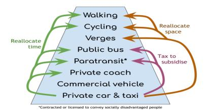
Putting the transport hierarchy into place involves reallocating existing road space. The Cambridgeshire plan (above) for reallocation of road space is a first step towards making the hierarchy applicable and workable, with spending targets for measures to develop active travel. This follows best practice and the example of many continental cities and towns<sup>13</sup>.
